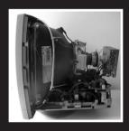
decided to open it, hoping it could be repaired. However, when I removed the cover I noticed that the narrow end of the glass tube was broken.
